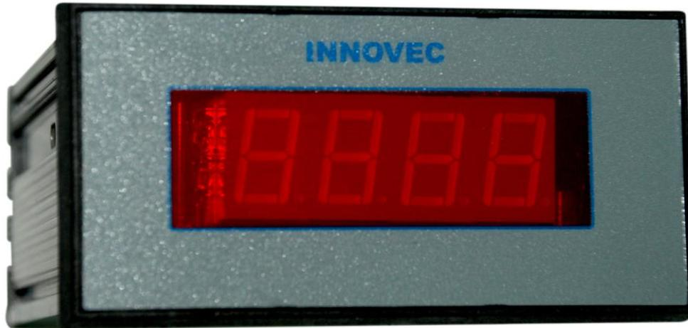
The **DI35 Powered Process Indicator** is a 120/240VAC or 9-36VDC powered 3.5 digit (1999 count) process indicator supplied in a panel mount enclosure with a 14.2mm high LED display which is range able in engineering units for millivolt, milliamp and voltage inputs. An optional 24VDC at 30mA loop supply is available for the direct connection of 2 wire transmitters.
