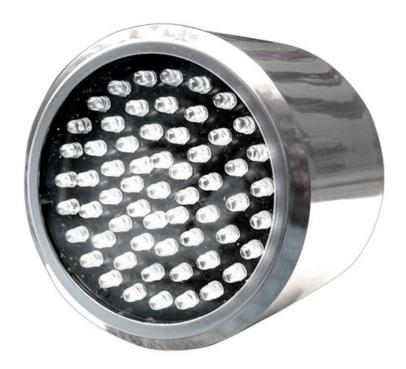
**The LEDML140 MARKER LIGHT** is a 24VDC powered LED ARRAY (60 LED [light emitting diode]) Marker Light supplied in a surface mount bright clear anodised enclosure with an IP65 weatherproof rating.
