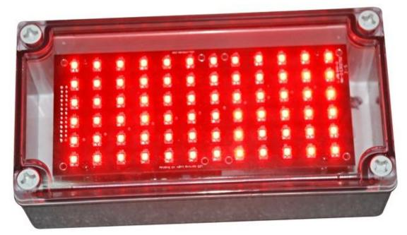
**The LEDHL SAFETY LIGHT** is a 120/240VAC or 24VDC powered LED ARRAY 72 LED [light emitting diode] warning light supplied in a surface mount enclosure with an IP67 weatherproof rating.
